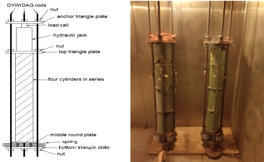
Fig. 2. Loading setup for environmental chamber
