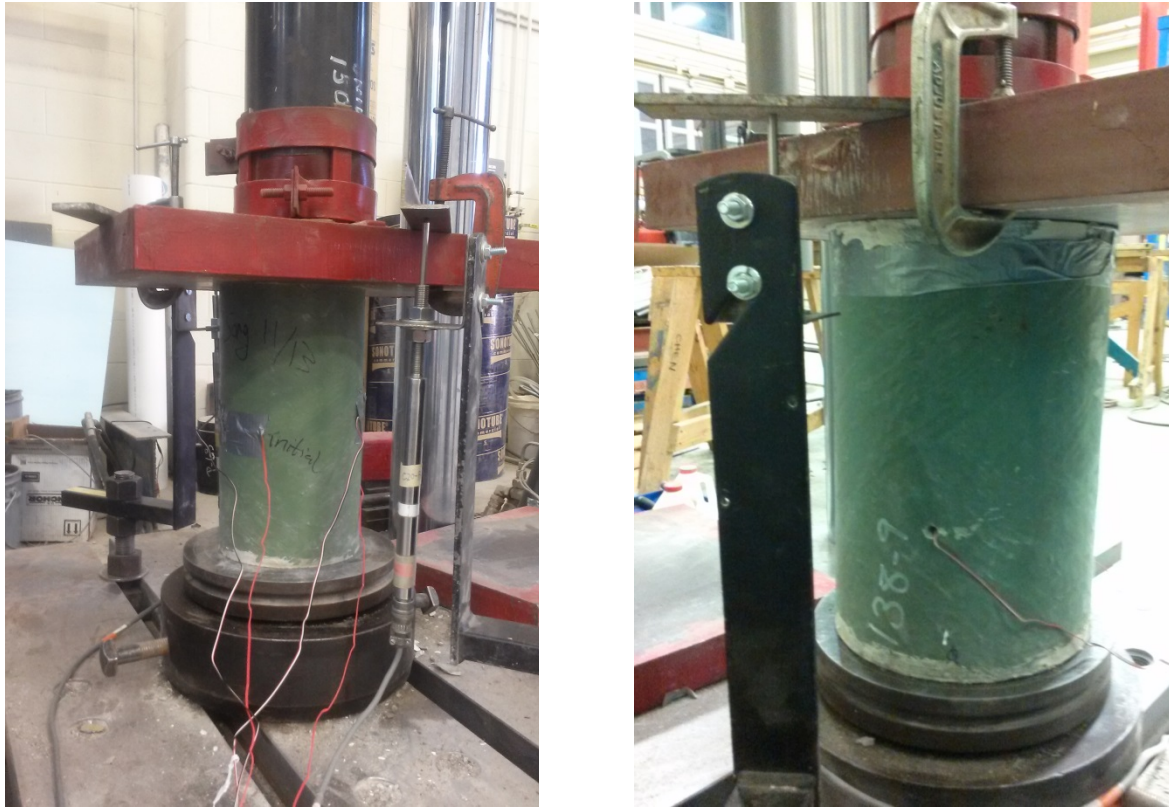
Fig. 4. (a) Setup for compression test on cylinders; (b) Tiny hole on the DST cylinder
